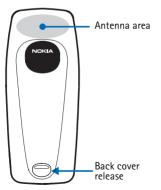
On the back of your phone, you will find the back cover release button. When you remove the back cover, you will find an antenna area, which is similar to the one shown in the graphic on the left.
