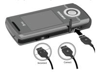
Note: The previous illustration shows both the correct method and the incorrect method for connecting the charger. If the incorrect method is attempted, damage to the accessory port can occur voiding the phone's warranty.
