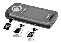
Push the microSD™ card into the slot until it clicks into place. Warning!: Make sure the printed circuit side of the microSD™ card is facing down when inserted.
