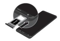
Slide the SIM card/Memory card tray back into the slot. **Note**: Your device is IP68 rated for dust and water resistance. To maintain the water-resistant and dust-resistant features of your device, make sure that the SIM card/Memory card tray openings are maintained free of dust and water, and the tray is securely inserted prior to any exposure to liquids. For more information, refer to "Maintaining Water and Dust Resistance" on page 200.
